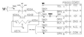
**NOTE:** For EC Fan DDC controller information and wiring, reference ED 19123.
