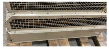
Figure 88: Side panel of hood (one on both sides) needed to be removed to secure hood
