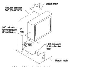
**5GA or 8GA coils.** Note that the addition of a vacuum breaker to permit the coil to drain during shutdown.
