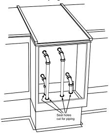
For units with standard base rails, the vestibule is open to the coil section; therefore, seal all holes to prevent air leakage.
