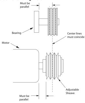
Figure 98: Adjustable Sheave Components
