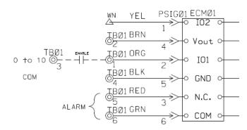
Figure 79: EBM Gen 3 Motor - Control Wiring with Manual/ Auto (Basic) Controls
