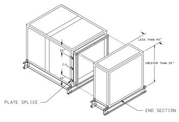
Figure 11: Splice Collar Alignment
