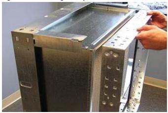
**STEP 6:** Place a latch so that the 2 tabs of the latch overlap the prefilter frame on each side of the corner. Slide the latch inside of the leg extension and align the latches' cap screw with the threaded coupling on the end of the leg extension and tighten using the hexkey. See Figure 29.
