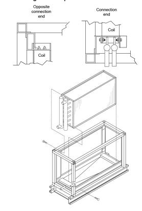
Figure 103: Single Coil Side Installation/Removal
