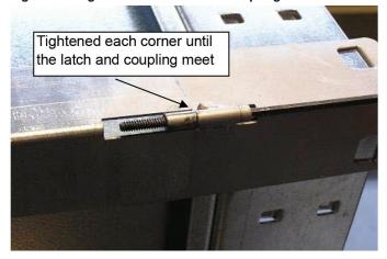
Once all four corners have been tightened the HEPA filter should now be properly seated and sealed.
