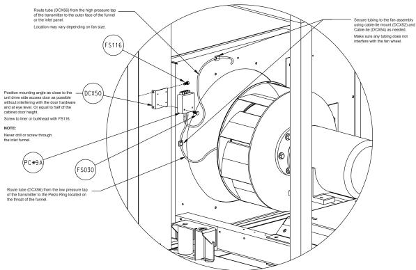
Figure 67: Fan Array Installation
