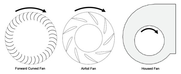
Fan wheel should rotate as shown
