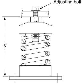
Table 4: Class II Belt-Drive Plenum Fan Spring Height
