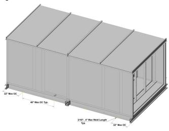
Figure 56: Unit with Base Frame Mounted on Concrete
