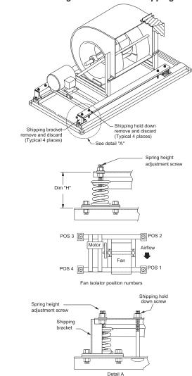
Figure 53: Plenum Fan Typical Shipping Brackets
