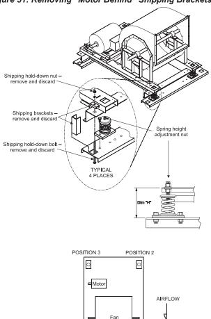
Figure 52: Removing "Motor Beside" Shipping Brackets
